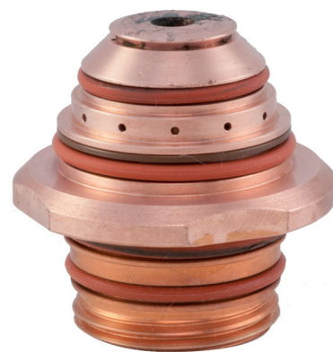
THERMACUT NOZZLE AFTER 6 HOUR CUTTING
