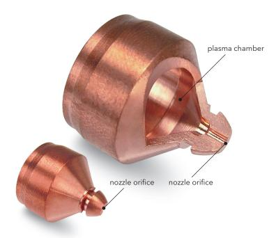
It is very important to maintain production precision of all consumables, particularly in the case of the nozzle orifice. Circularity, cylindricity, and roughness of the machined hole are factors that must be accounted for when the nozzle orifice is manufactured.
