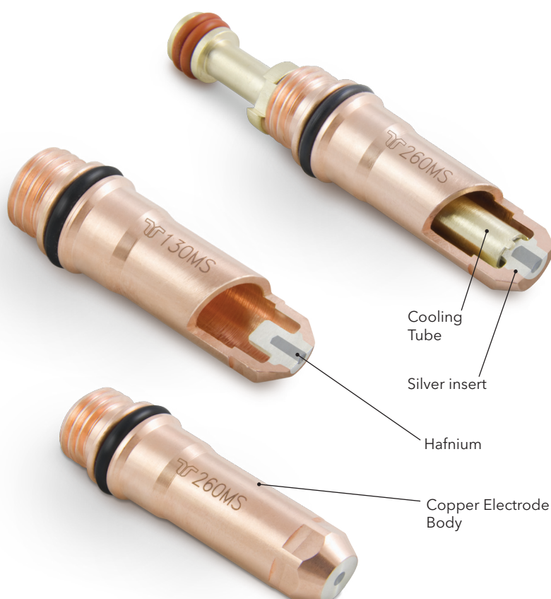
Pict. No. 1: Construction of the Silver PRO electrodes
