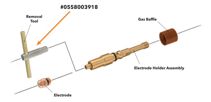
**NOTE:** Before assembling please apply a thin film of silicone lubricant (our ref. No. T-0994) on all o-rings to avoid leakage.
